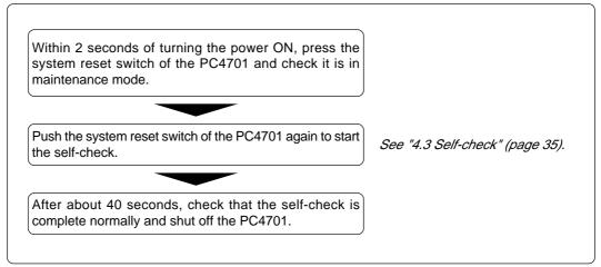
Figure 2.3 Self-check procedure
